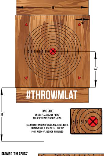
DRAWING "THE SPLITS" Extend a pencil guide line from the outer Most Ring Horizontal and vertically until the Guiders meet at the corners. Extend another guide line from the center of the Bullseye to the corner created by the Guides
